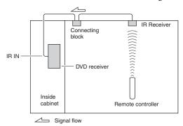
The miniplug cable from the connecting block should be connected to the DVD receiver's IR IN jack, as shown below.
